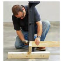
**TIP:** Use a scrap piece of wood for assembly support
